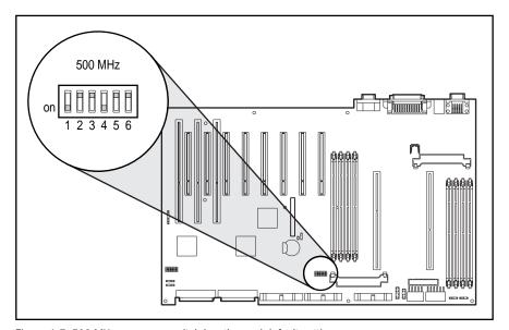
Figure 4-7. 500 MHz processor switch location and default setting
